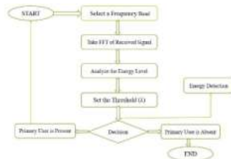
Figure 2 Flowchart for Proposed Spectrum Sensing for Cognitive Radio using Energy Detection
